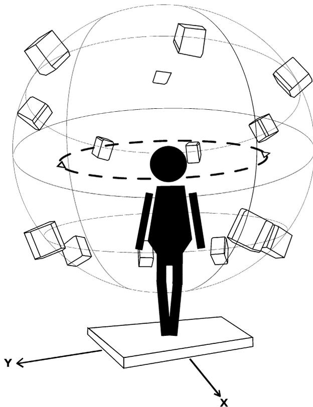
**Fig. 1** Experimental apparatus: The subject, who is standing on a force platform, is surrounded by the 16 loudspeakers of the Ambisonic system. The *dashed line* represents the simulated trajectory of the stimuli
