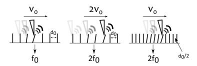
**Fig. 1.** A simple example of the phenomenological model of friction sounds. The three cases presented illustrate the ambiguity between velocity and roughness in the produced friction sound.
