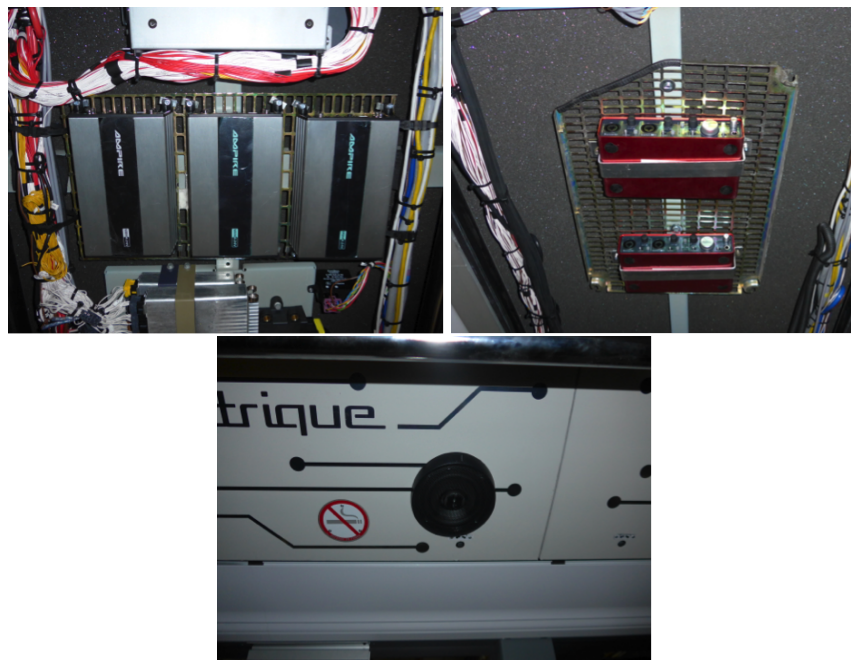
Fig. 2. Fixation of the amplifiers (top left), the sound cards (top right), and the loudspeakers (bottom).
