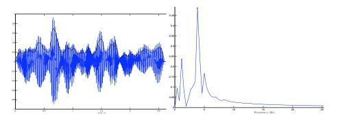
**Fig. 3.** <u>Left</u>: Estimation of the temporal envelope of a sound in the category "Rotate". Right: FFT of adjusted autocorrelation and extraction of peaks for the characterization of amplitude modulation of the temporal envelope. The selected peaks are marked by circles.
