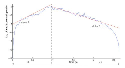
**Fig. 4.** Example of the Characterization of level variation for a sound from the category "go past" by the 2 slopes  $\alpha_1$  and  $\alpha_2$  of the interpolation process. The duration  $t_1$  (from the beginning of the signal to its max value) and  $t_2$  (from the max to the end) were also considered.
